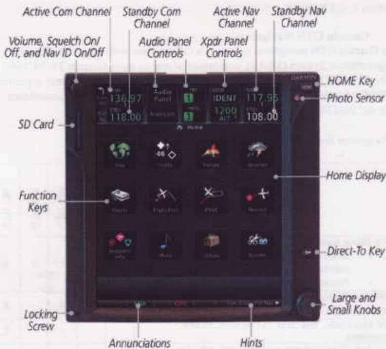
Figure 1 - GTN 750 Control and Display Layout
